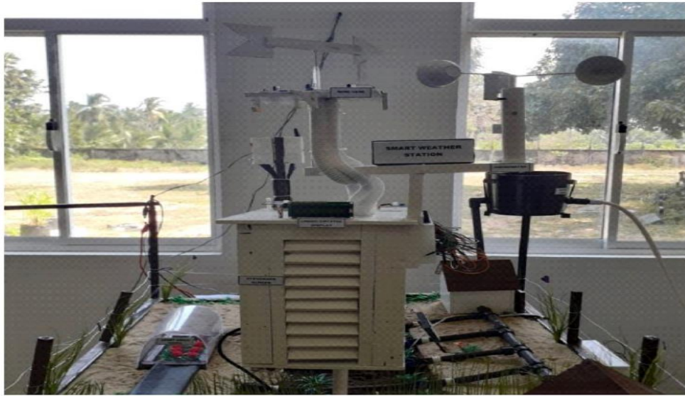
Figure 2.10: Shows the Smart Weather Monitoring System
