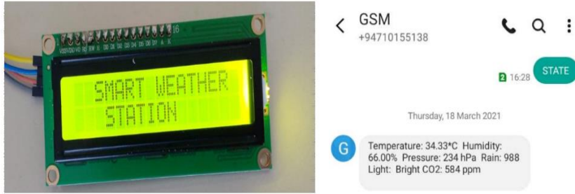
Figure 2.9: Shows the Output Unit of the Smart Farming System
