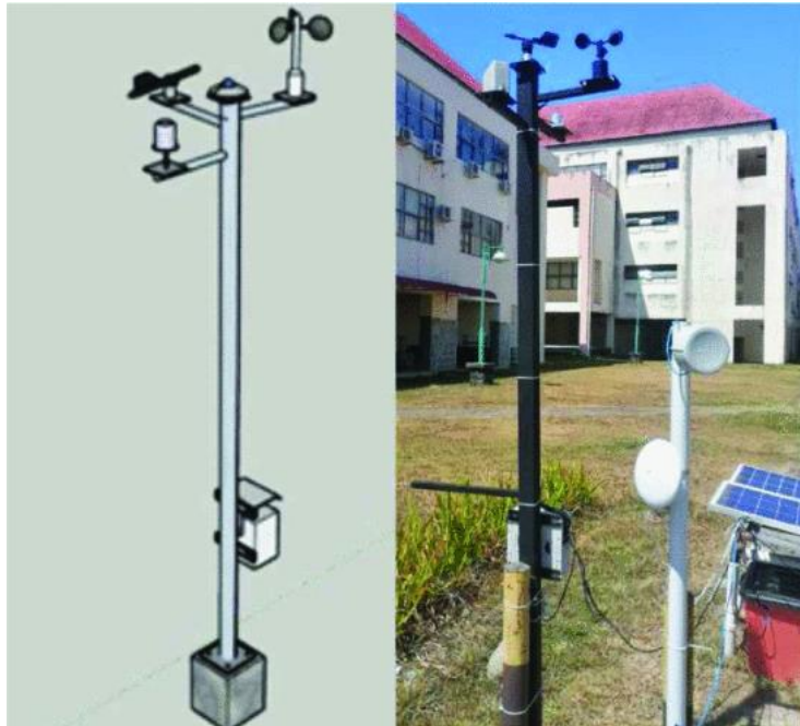
Figure 2.4: Shows the 3D Design of Weather Station along with actual on-site Installation of Structure
