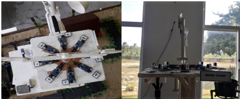
Figure 2.11: Shows the Low-cost Wind Vane of the Smart Farming System
