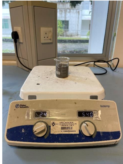
GNPs powder being stirred in ethanol solution using magnetic stirrer
