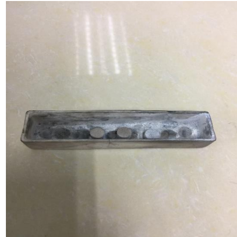
Fabricated samples after sintered in the tube furnace
