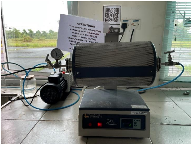
Tube furnace with argon gas environment
