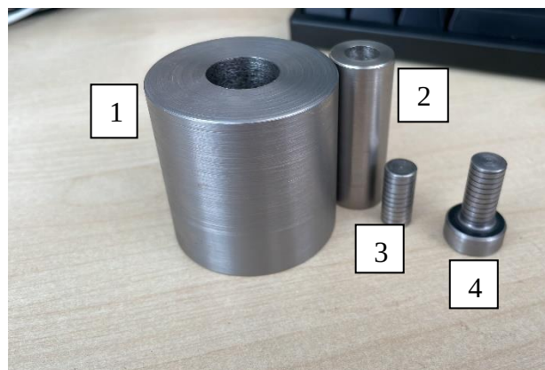
Sample compactor for powder metallurgy: consist of 1) Body 2) Die 3) Stopper 4) Compactor
