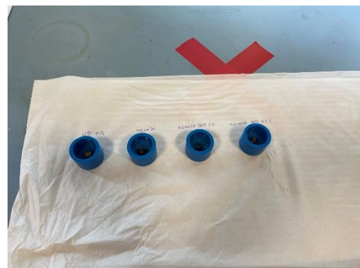
Samples are prepared to be mounted using epoxy resin
