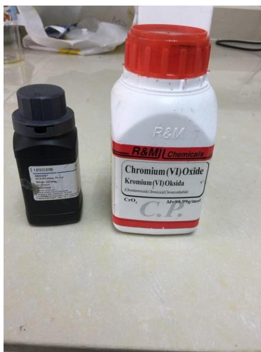
\text{Cr}_2\text{O}_3 and \text{AgNO}_3 used for cleaning samples to remove corrosion products
