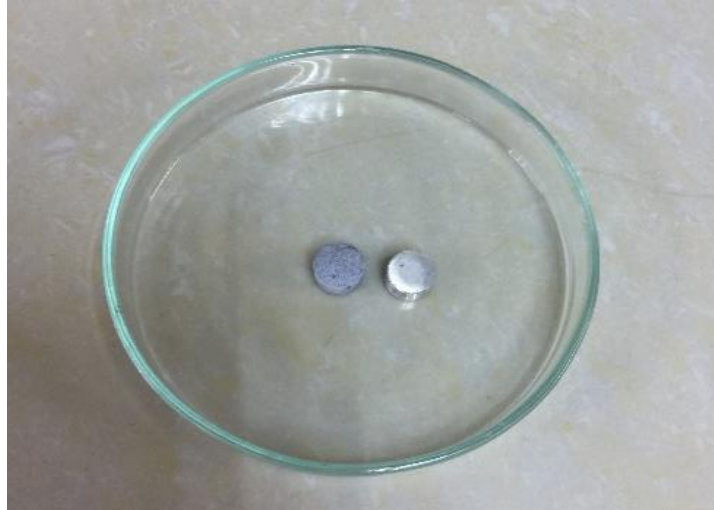
Figure 3.2: Fabricated HP Mg sample before polish and HP Mg samples after polish
