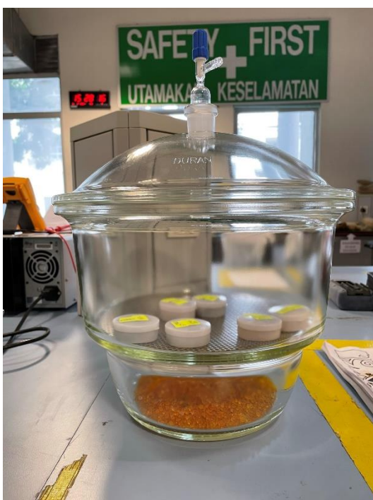
Dessicator used for store samples after immersion test
