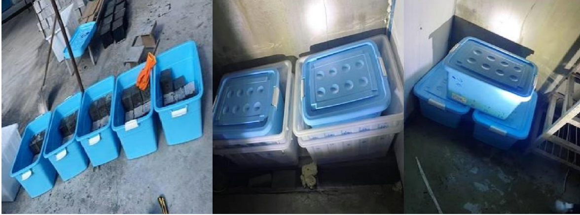
Figure 3.7: Immersion of Concrete Test Blocks
