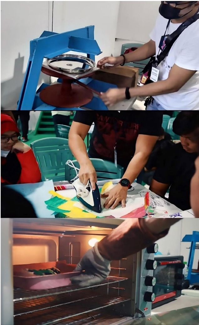
FIGURE 3 | Participants learning and practicing HDPE plastic processing techniques during the co-creation workshop, including oven melting and ironing processes (Source: Personal Photograph, 2022). [Color figure can be viewed at wileyonlinelibrary.com ]
