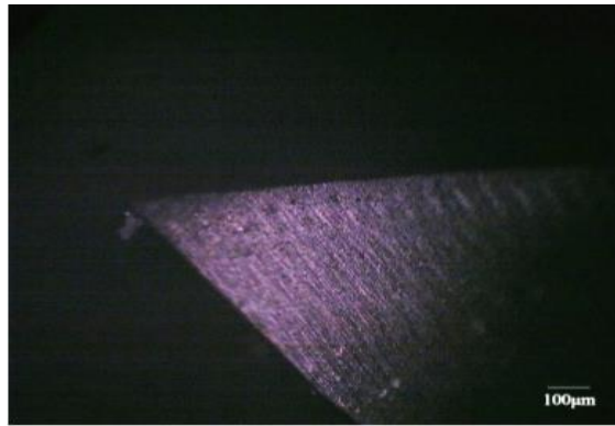
Figure 4.32: Tool edge on new cutting tool (Before cutting process).
