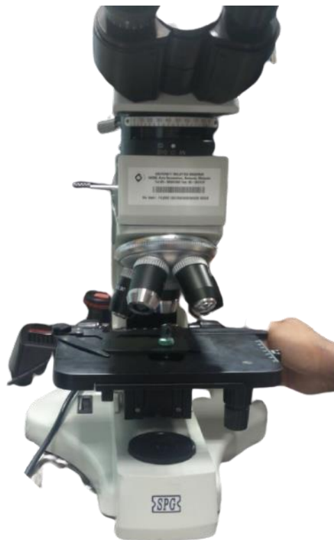
Figure 3.18: SPG optical microscope 100X
