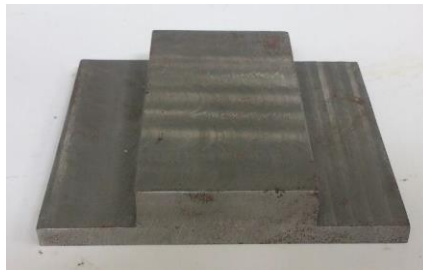
Figure 3.13: Shape of AISI 1095's work material
