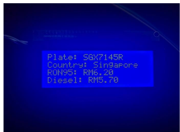
Figure 4.3 LCD showing detected Singapore plate with fuel pricing.
