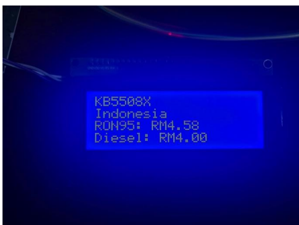
Figure 4.2 LCD showing detected Indonesian plate with foreign pricing
