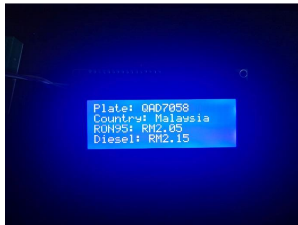
Figure 4.1 LCD showing detected Malaysian plate with subsidised pricing.
