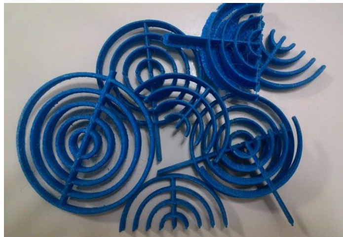
Figure 32: Printed lantern wind turbine after surface finishing
