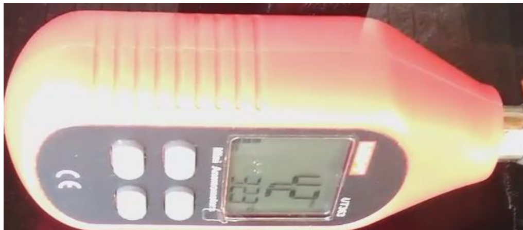
Figure 47: Speed measurement velocity 4.2 m/s (pictures obtained from experimental video)
