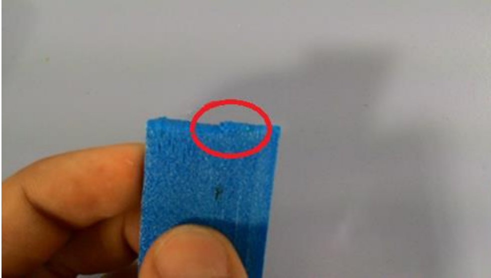
Figure 26: Distorted model with shaking of platform
