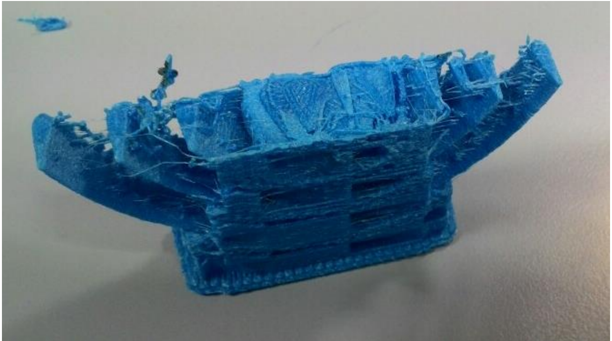
Figure 28: Designed failed to be printed.
