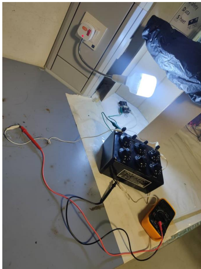
Figure 4.2: DSSC Set Up
