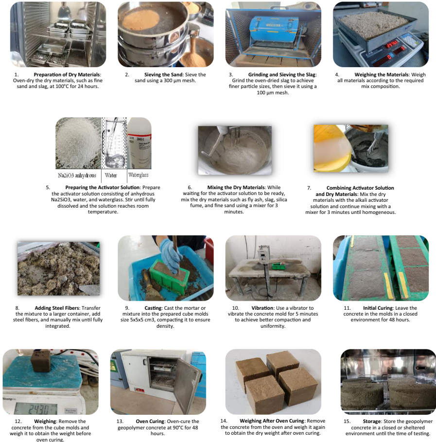
Figure 14.4 Steps for geopolymer concrete production.
