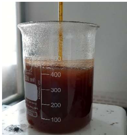
Figure 3.4: Powdered SPW in 4% w/v NaOH Solution
