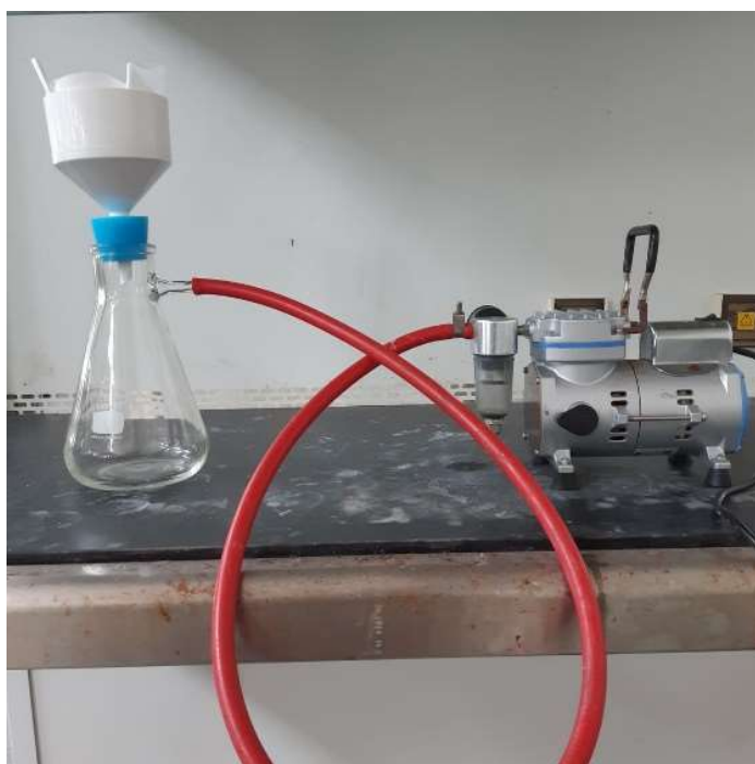
Figure 3.5: Buchner Funnel, Buchner Flask, and Vacuum Used for Filtering Process
