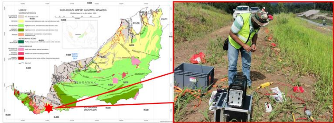
Figure 3.8: Electrical Resistivity Tomography for Site-Specific Suffusion Assessment
