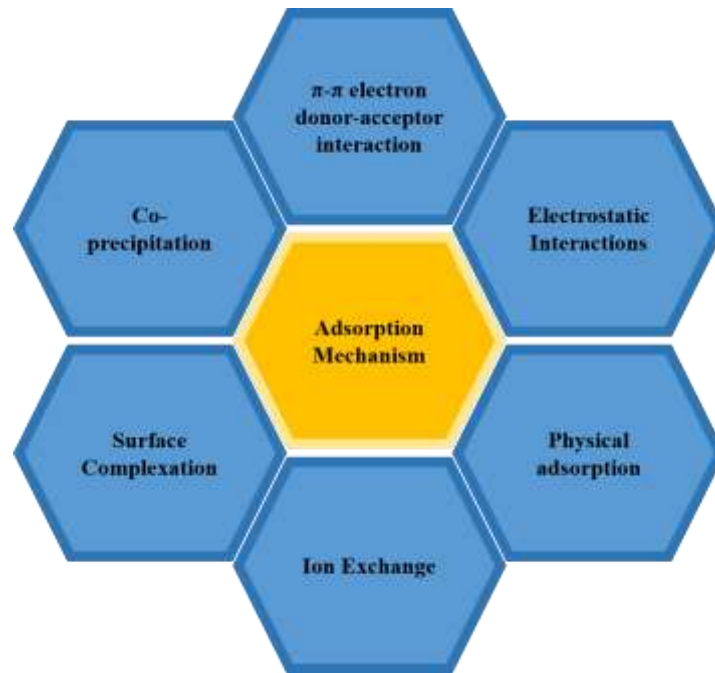
Figure 2.1: Heavy metal removal mechanism by adsorbent (Shakoor et al., 2020; Liu et al., 2020)
