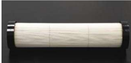
Figure 2.2: Ceramic hollow–fibre membrane (Samaei et al., 2018).
