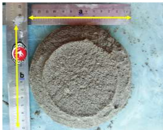
Figure 3.14: Foamed concrete slump measuring
