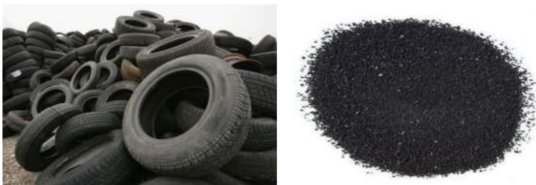
Figure 2.16: Scrap tire is crumbled into powder for casting in concrete
