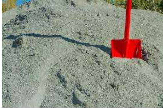
Figure 3.20: Quarry dust used in foamed concrete production
