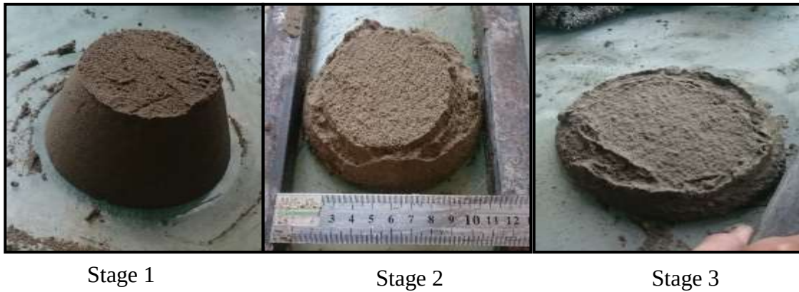
Figure 4.11: Three stages of slump
