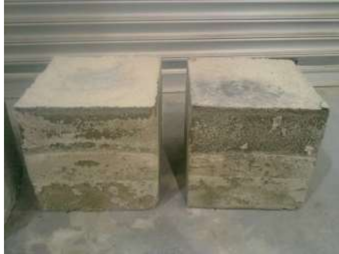
Figure 6.1: Foamed concrete block produced in three-layer by using conventional mixing technique
