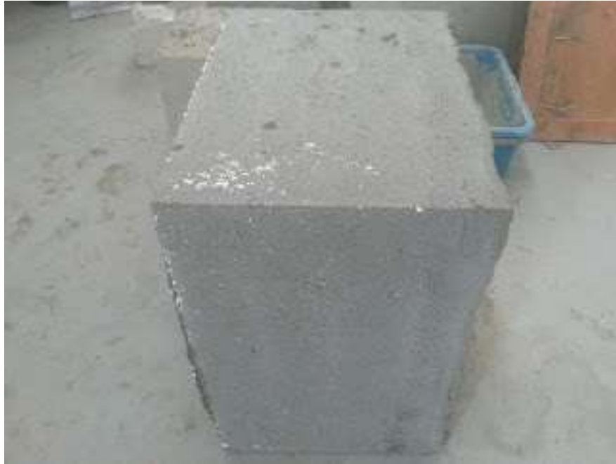
Figure 6.2: Foamed concrete block produced by new mixing technique with minimised shrinkage
