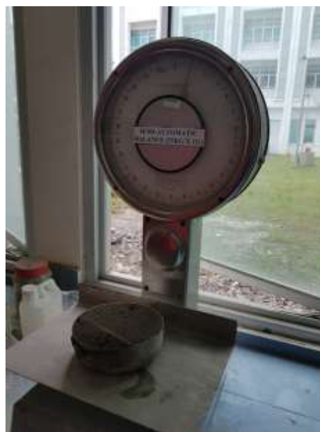
Figure 3.15: Foamed concrete density measurement
