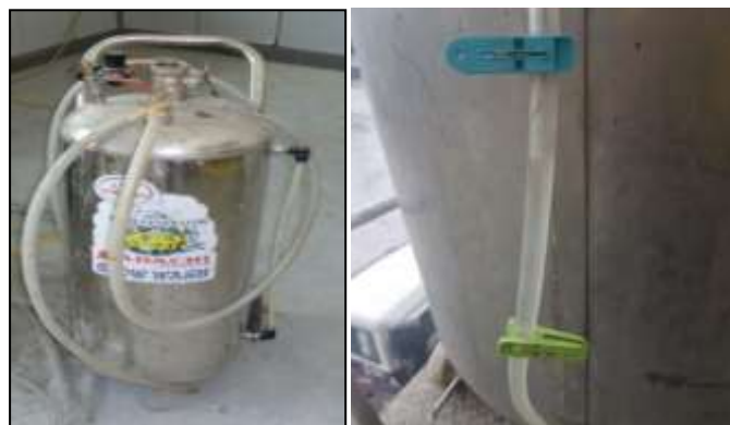
Figure 3.12: Equipment used to produce foam and measure the volume of foam
