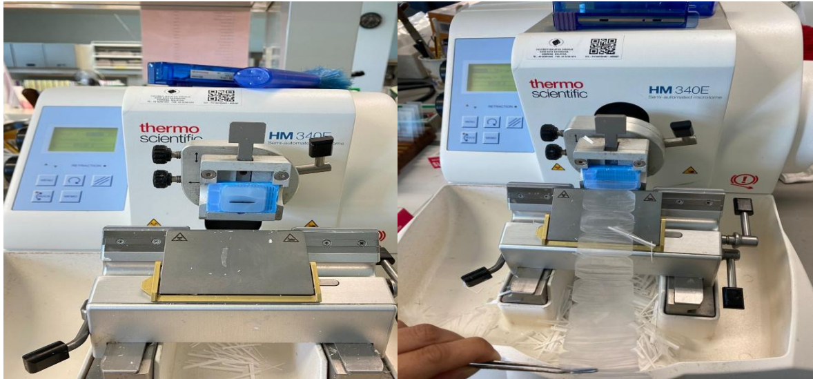
Figure 3.18: Semi-automatic microtome machine used for trimming and sectioning.
