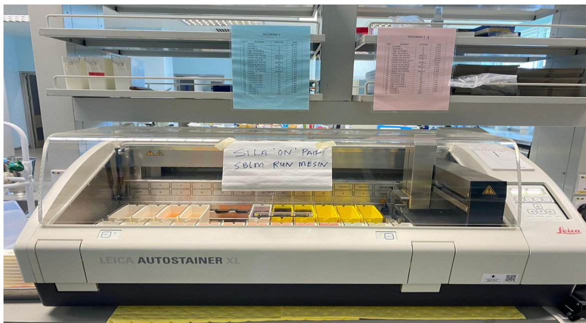
Figure 3.20: Leica Auto stainer XL used for Haematoxylin and Eosin (H&E) staining.
