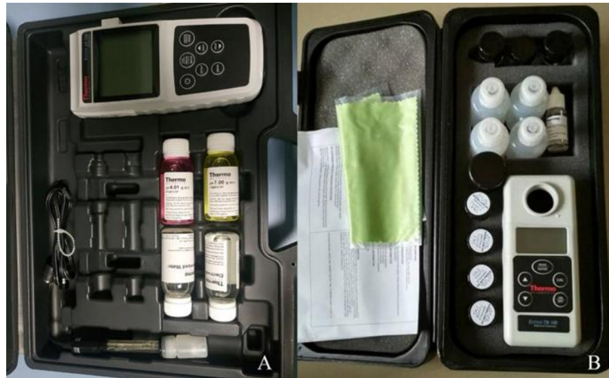
Figure 3.12: A - pH meter, Eutech pH 150 and B - waterproof handheld turbidimeter, Eutech ECTN 100 IR.
