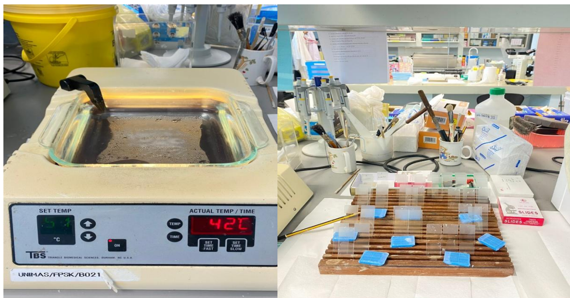
Figure 3.19: Floatation bath used for skin fishing along with the slides containing skin samples.
