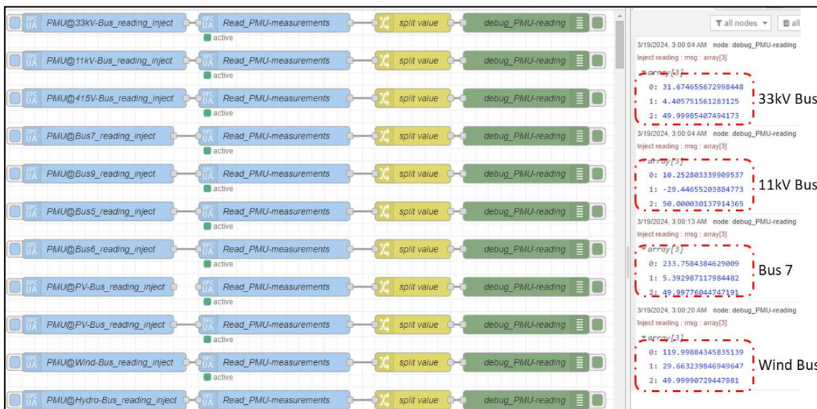
Figure 4.6: PMU Measurements Published in Node-RED Interface
