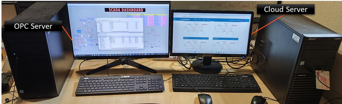
Figure 2: Laboratory Experiment of Phasor Data Sharing in WAMS
