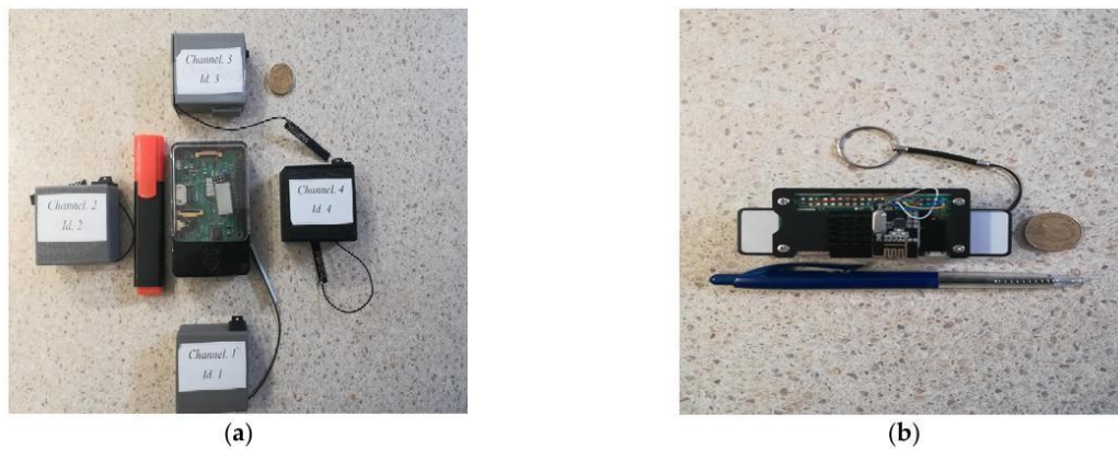
Figure 2.6: a) RPi3B as a base station gateway, (b) RPiZW as a portable gateway (Al-Naime et al., 2023).
