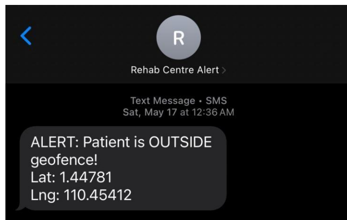
Figure 3.11: SMS notification system when patient is outside the rehab center geofence.
