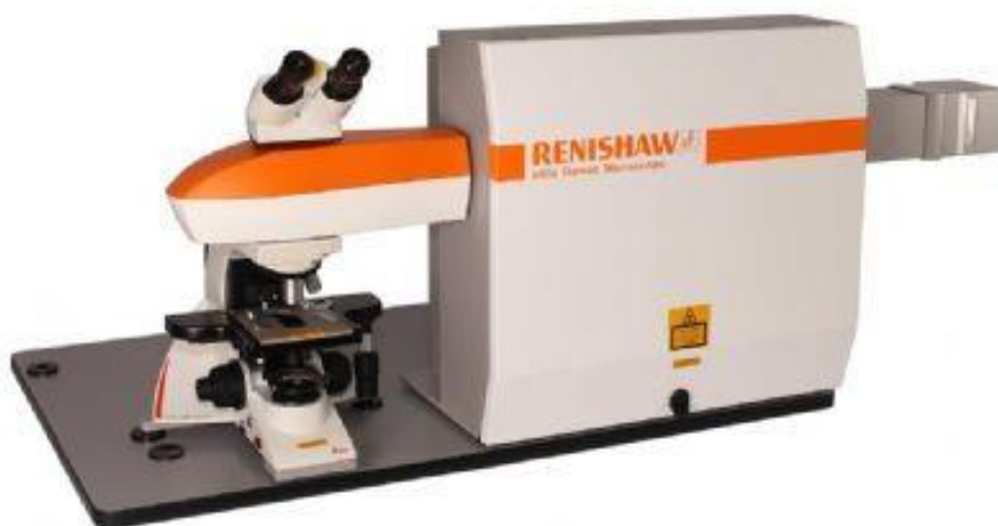
Figure 7: Raman Spectrometer (InVia Reflex, Renishaw, UK)
