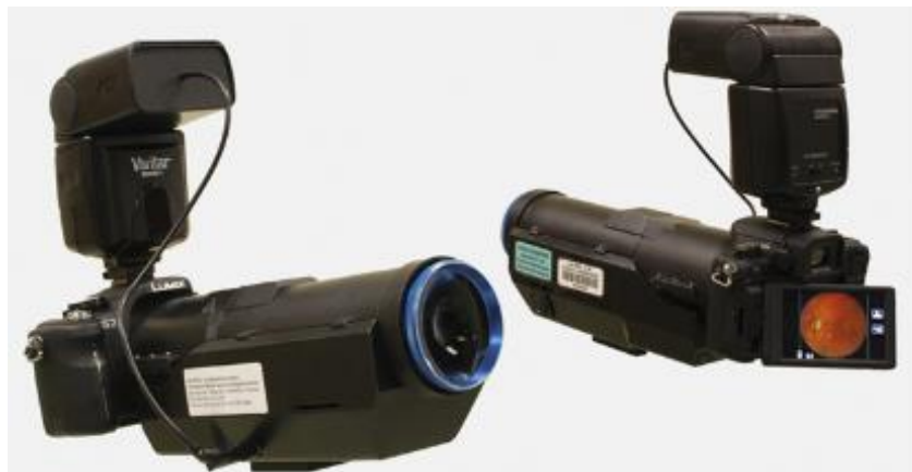
Figure 2.8: Front and rear view of the developed handheld fundus camera prototype (Tran et al., 2012)
