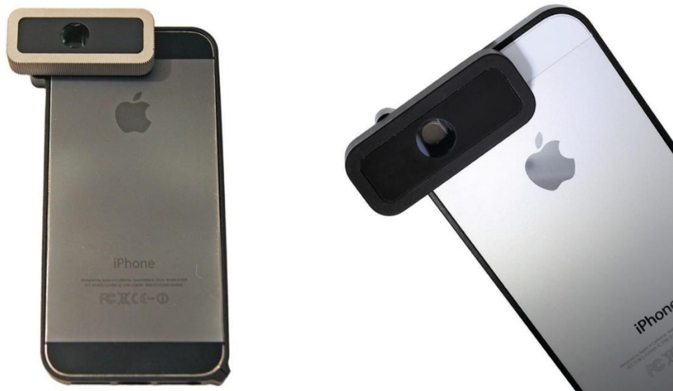
Figure 2.9: D-Eye prototype attached to an iPhone 5 and iPhone 5s from the left (Russo et al., 2015a)
