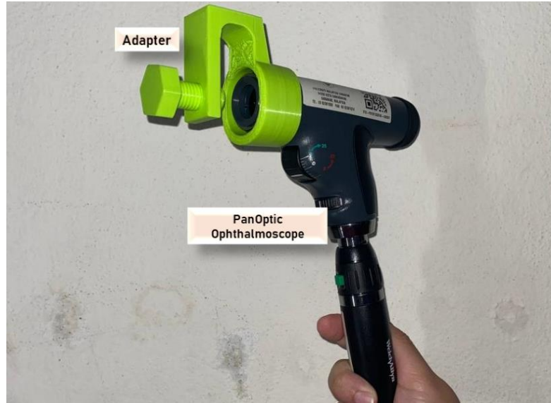
Figure 4.4: Printed second prototype when used with Pan Optic
