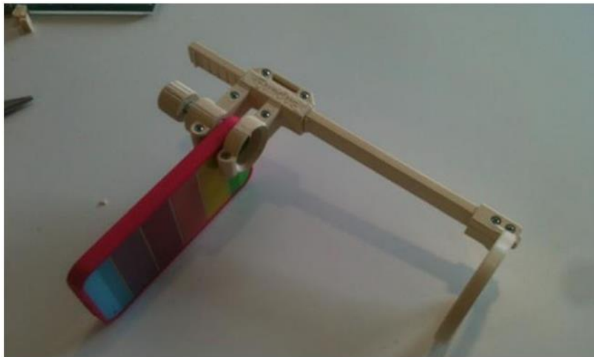
Figure 2.10: 3D-printed retinal image acquisition adapter (Hong, 2015)
