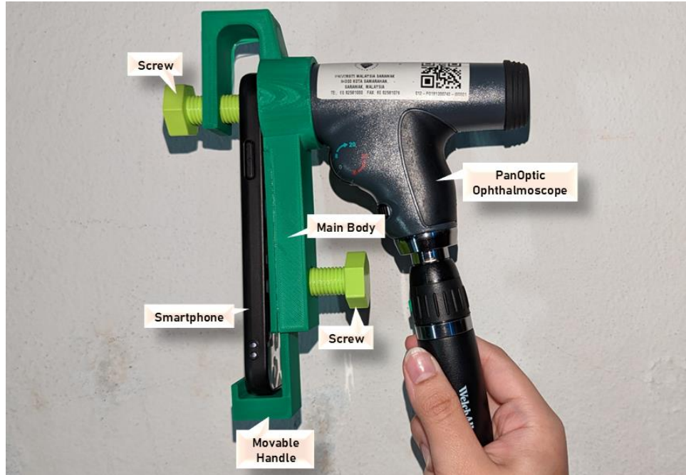
Figure 4.6: Printed third prototype when used with Pan Optic and smartphone
