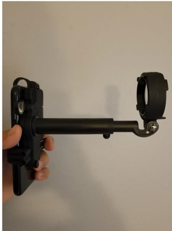
Figure 2.13: Side view of the Paxos Scope used with an iPhone (Mercado et al., 2017)
