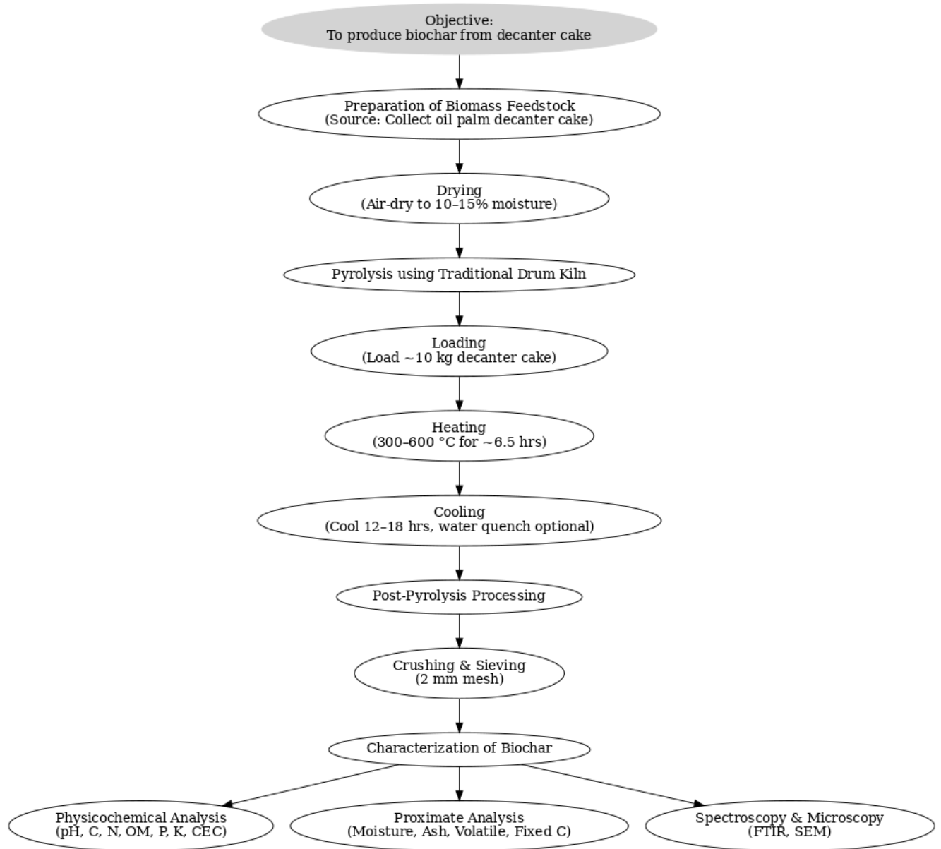
Figure 3.1: Sequential processes involved in the preparation and characterization of biochar from oil palm decanter cake.
