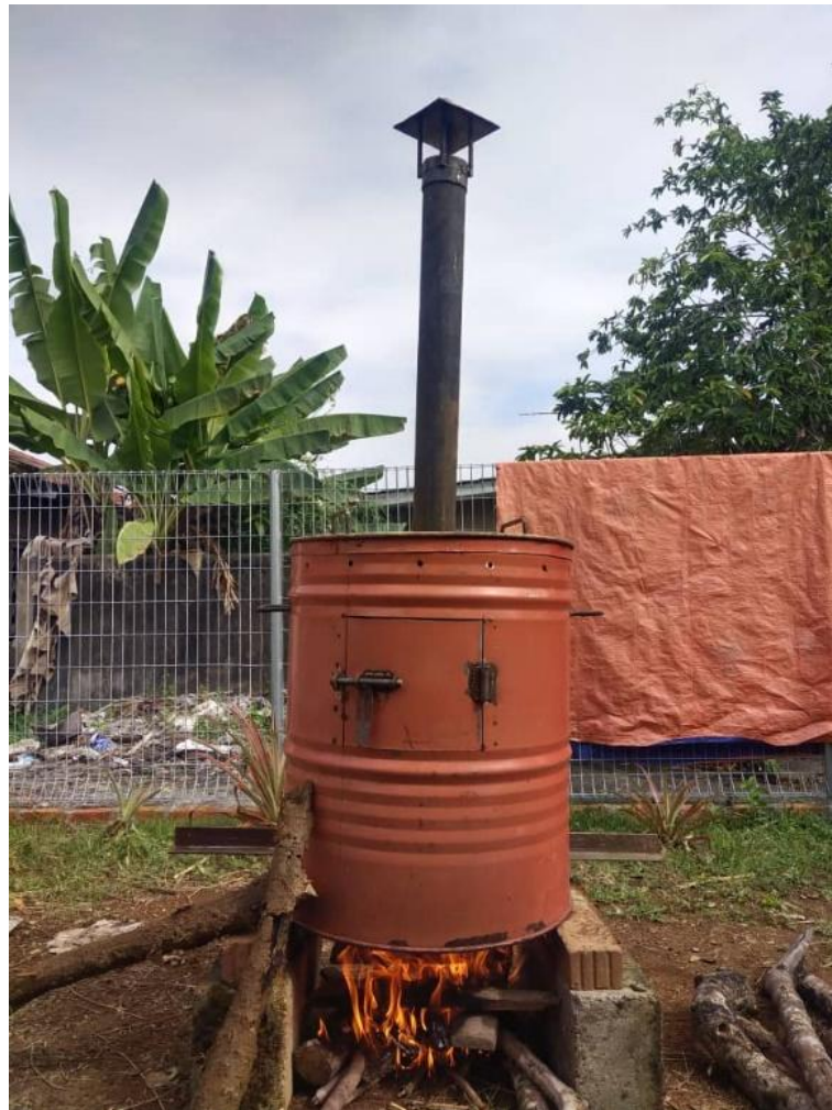
Figure 3.2. Preparation of biochar using a modified drum kiln. The feedstock is heated under limited oxygen conditions to produce carbon-rich biochar. (Image by Deborah Renting Jimmy, 2025)
