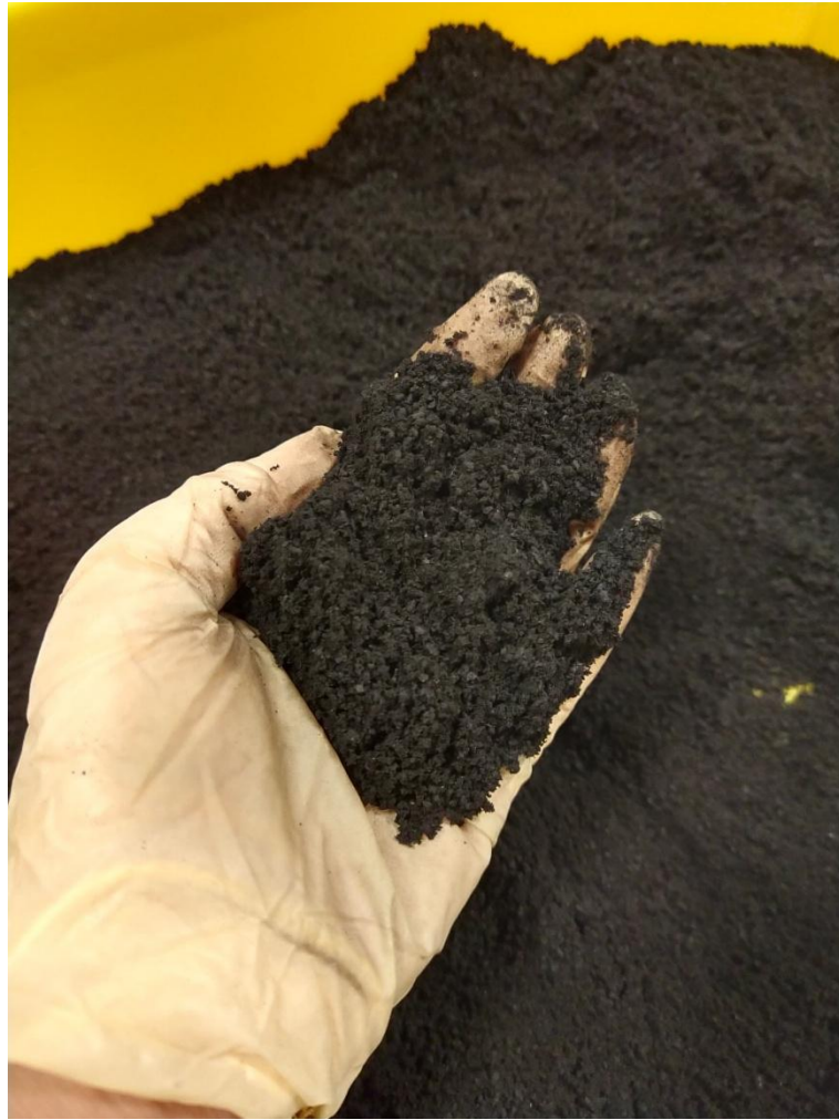
Figure 3.3. Biochar was produced from decanter cake via pyrolysis using a traditional drum kiln (Image by Deborah Renting Jimmy, 2025)
