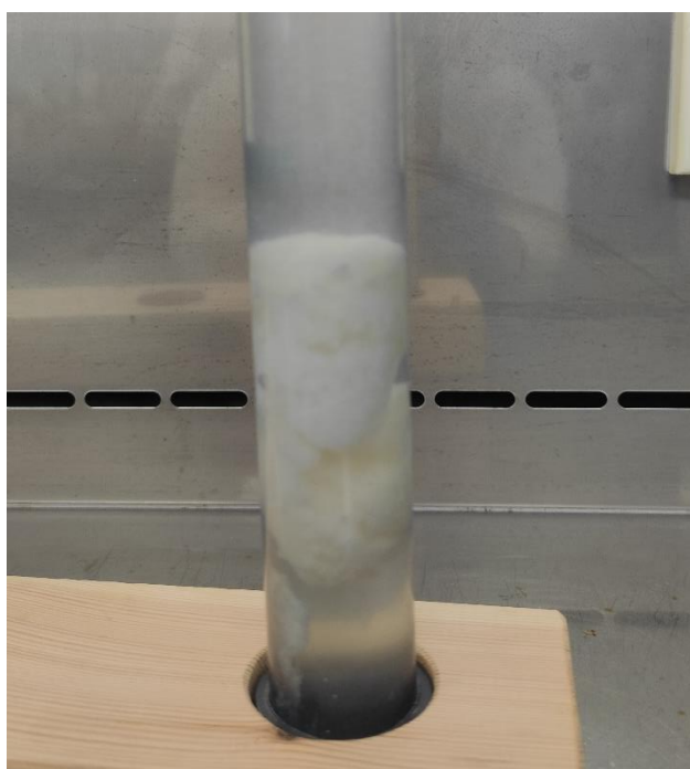
Figure 4.3 Snapshot of precipitation formed from direct mixture of digested solution (KOH) and density separation medium ( \text{ZnCl}_2 ).
