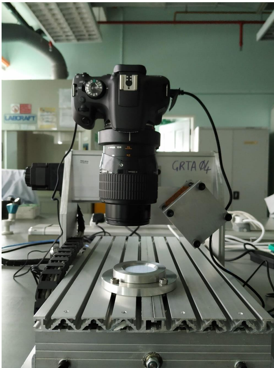
Automated filter-scanning rig
