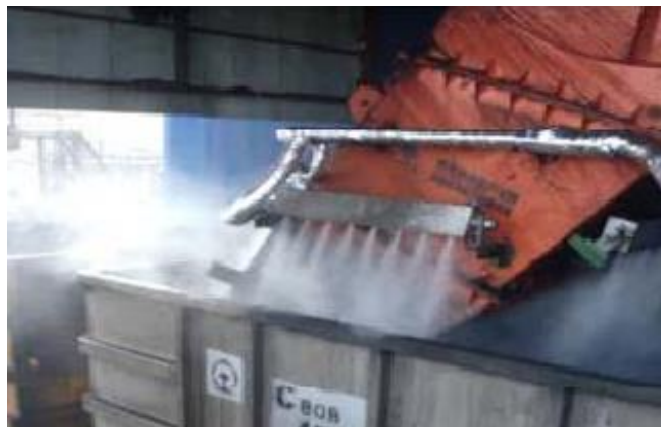
Figure 2.2: Fine water mist dust removal (Zhou & Qin, 2021)
