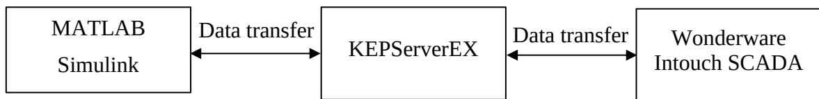
Figure 3.25: Data Transfer between MATLAB Simulink and SCADA
