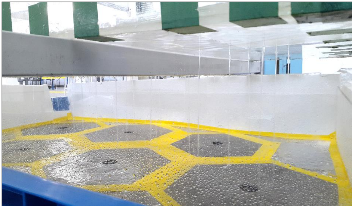
Figure 3.22: Simulating the Rain Intensity through Tiny Holes
