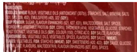
Figure 32. OCR failure due to reflective packaging
