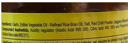
Figure 31. OCR failure due to shape of the packaging
