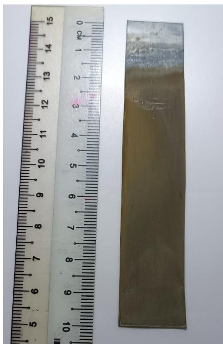
Figure 4.15: Surface condition of ZnO/Zn photoanode in 100% POME solution after 8 th hour
