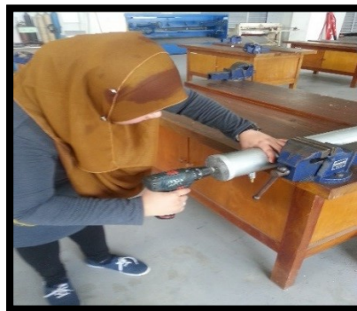
Figure 3.2: Drill Holes into the Ruben's Tube
