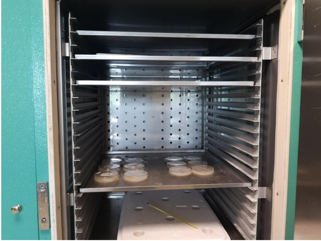
Figure 3.1: Germination experiment in unlit incubator (Convion G30 Model, Winnipeg, Canada).
