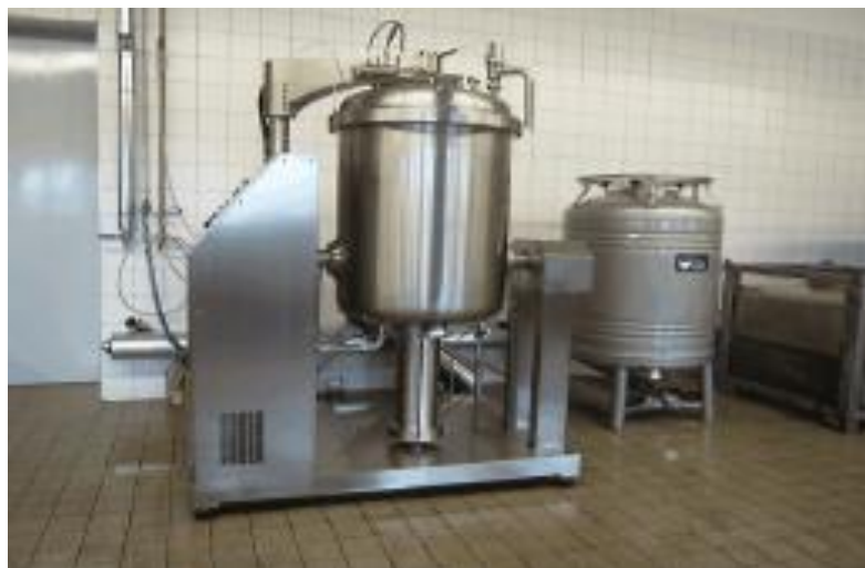
Figure 2.7: A solvent extraction unit that combined with distillation process for agarwood oils extraction (Pakamas, 2012)
