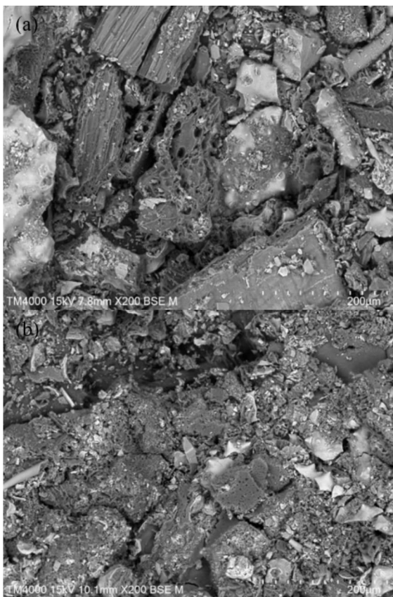
Fig. 2 Surface morphology of (a) uncoated and (b) corn starch/soybean wax coated biochar-based fertilizers (200 \times magnification)
