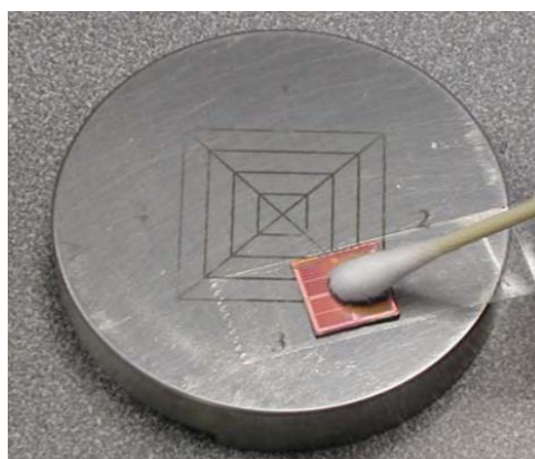
Figure 3.9: Use cotton swab to pressure the die down to make sure stick firmly
