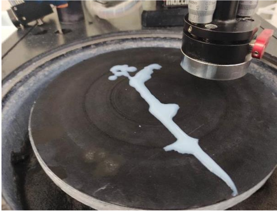
Figure 2.14: Parallel lapping pad with colloidal silica suspension slurry
