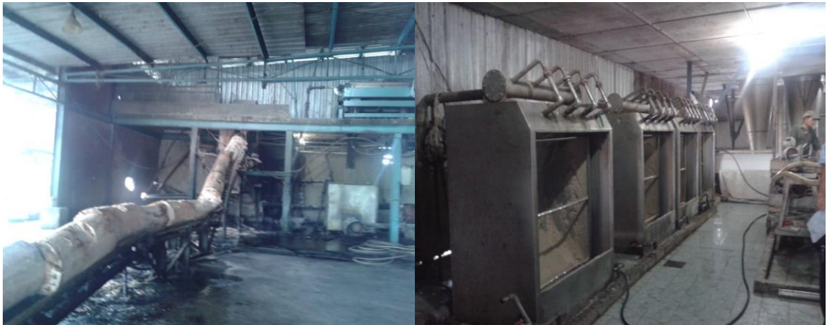
Figure 1.5: Debarked sago logs were mashed into a rasper (left) and water is added to form starch slurry (right).
