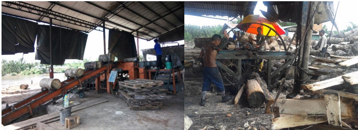
Figure 1.4: Sago logs were debarked automatically by using automated machine (left) or manually by human (right).
