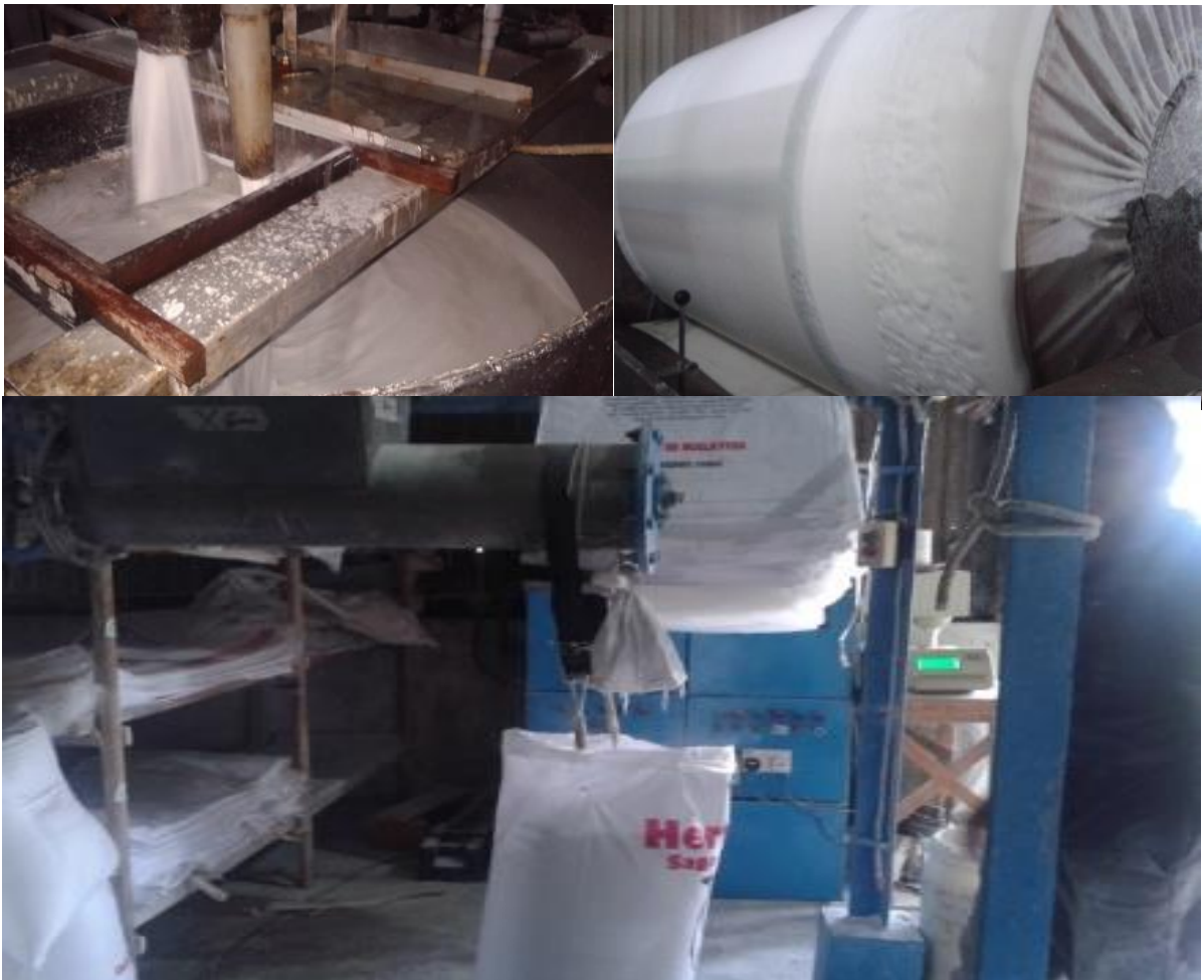
Figure 1.6: Starch slurry is allowed to settle down in the tank, dry and finally form sago flour that are ready for packaging.
