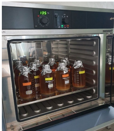
Figure 3.8: Thermal ageing using Thermal Oven
