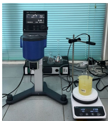
Figure 3.13: Heating of POME-based TiO 2 -ZnO HNF using magnetic stirrer at 40 °C
