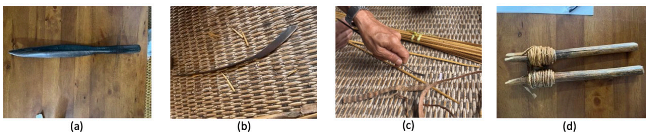
Figure 4: a) Sosag, for pushing tree bark into the weaves, b) Sindak pait a sharp blade for cutting, c) Kiru, a metal tool to untuck the weaves, d) A pair of sticks to tie the edge of kasah
