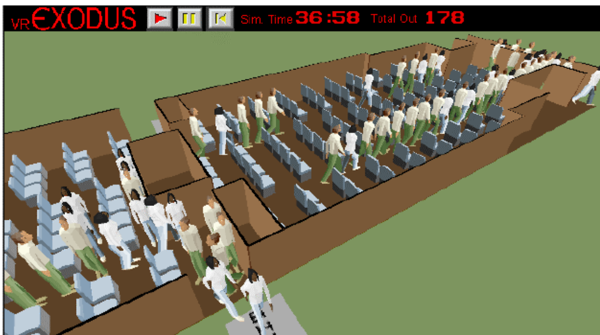
Figure 9: Example scene using Exodus for evacuation simulation
