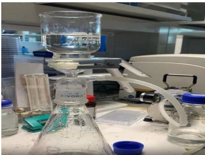
Figure 3.1: The Setup for Degassing Solvents A and B Using Vacuum Filtration Apparatus The assembly involves connecting a filter flask with a vacuum adapter to a vacuum pump via tubing. Filter paper is placed in the funnel, wetted with solvent, and the mixture to be filtered is poured into the funnel. Suction created by the vacuum pump pulls the liquid through the filter paper, and the filtrate is collected in the flask.
