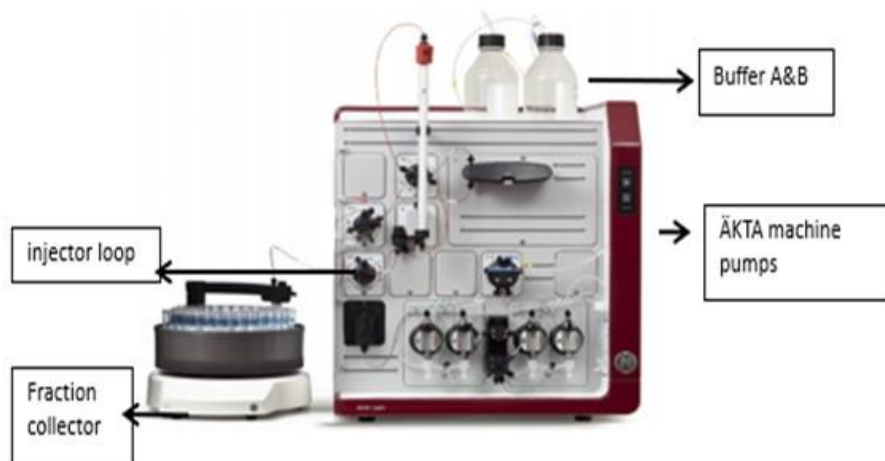
Figure 3.5: ÄKTA Pure™ Chromatography System integrates essential components for efficient chromatographic separations. This includes a pump module, injector valve loop, a UV detector and a fraction collector for collecting eluted fractions.
