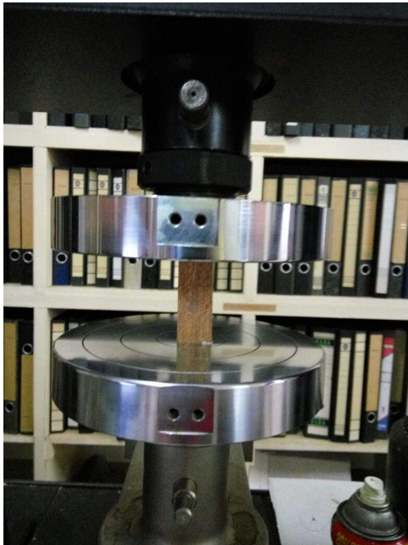
Figure 3.1: Compression parallel to grain test.
