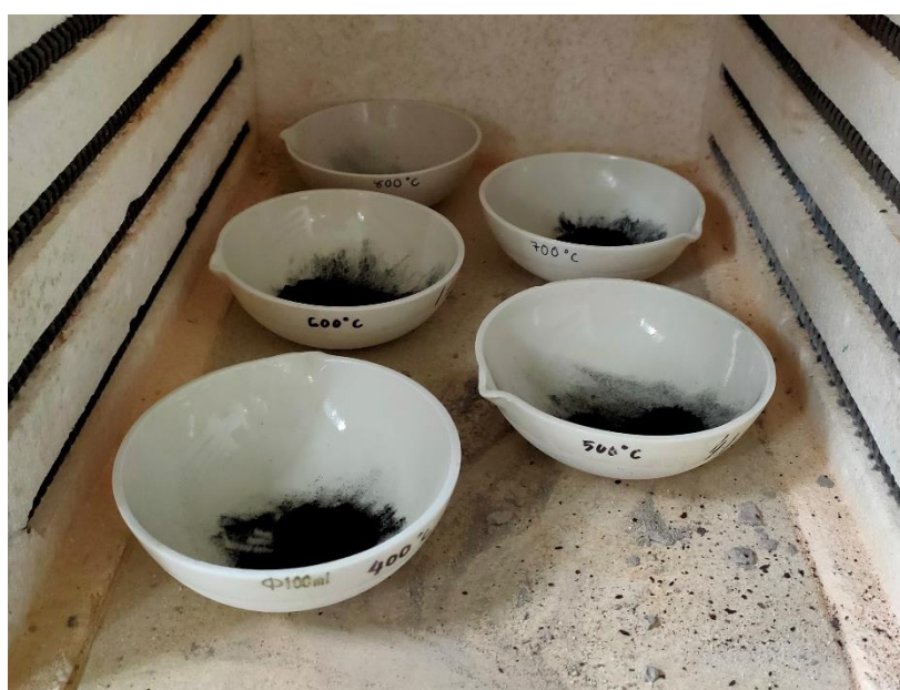
Figure 3.7: Ash content determination.
