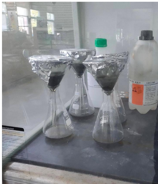
Figure 3.7: Chemical activation of biochar using chemical activating agents, performed in fume hood.
