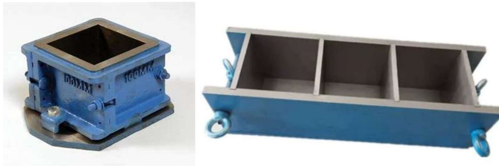
Figure 3.1: 100*100*100mm Cast Icon Mold, Single and Tri-slots
