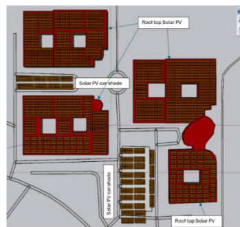
Fig. 8. Digital model of FK buildings- site plan view featuring roof solar PV and solar PV car shade.
