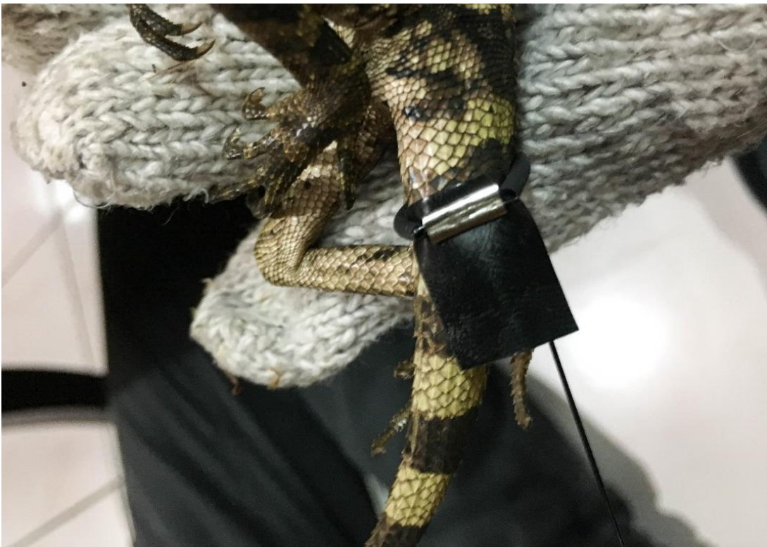
Figure 3.2: Taping electric tape around the compressed crimp sleeve and cut wires
