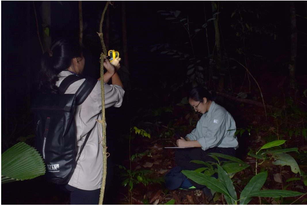
Figure 5.1: Measuring surface body temperature, T_b and perch surface temperature, T_s using a handheld infrared laser thermometer (Fluke 62 MAX)
