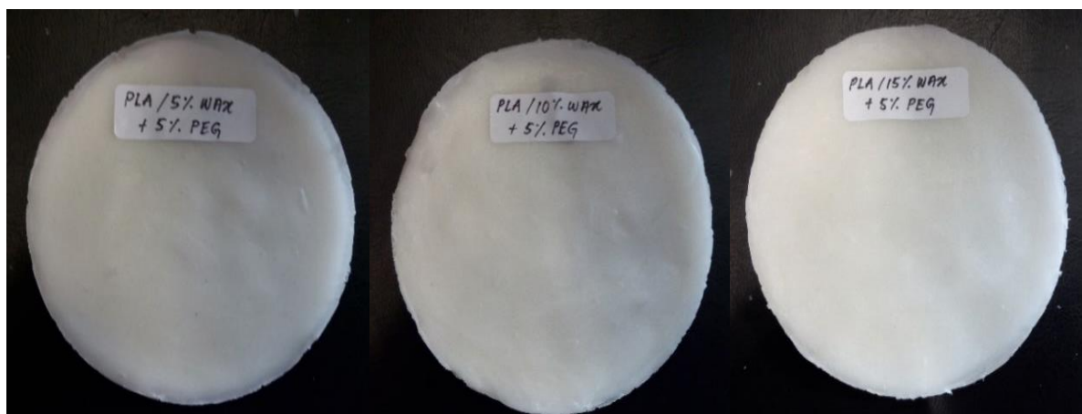
Figure 4.2: PLA/wax composites prepared by melt blending method with different wax loading. (a) PLA/wax composite (95/5/0) with no addition of polyethylene glycol (PEG), (b) PLA/wax composite (95/5/5) with the addition of 5 wt.% PEG, (c) PLA/wax composite (90/10/5) with the addition of 5 wt.% PEG, (d) PLA/wax composite (85/15/5) with the addition of 5 wt.% PEG
