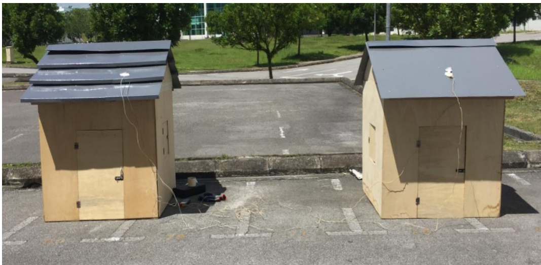
Figure 3.5: On-site experiment for small-scale model house with ventilated roof (left) and common roof (right)
