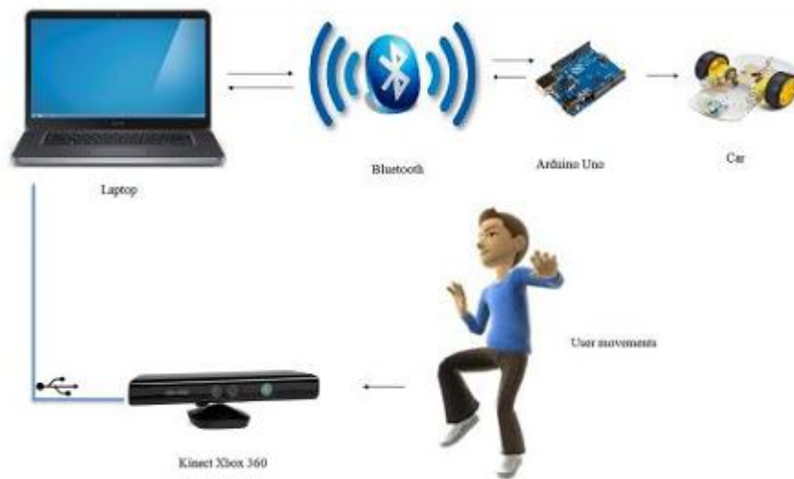
Figure 7: System Architecture for Gesture Control of a Mobile Robot using Kinect Sensor
