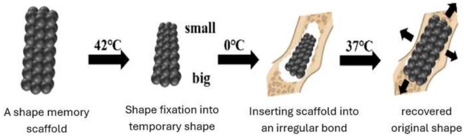
Figure 11.2 Illustration of shape memory scaffold process. The process of a thermo-responsive shape memory scaffold implementation for an irregular bone defect area by PLLA-TMC-GA and PHA scaffold.
