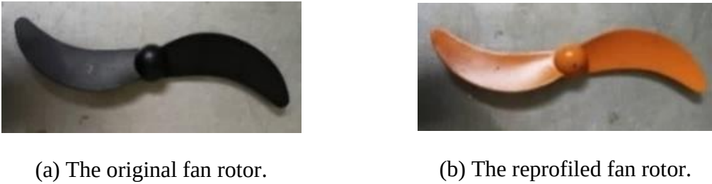
Figure 3.45: The fan rotor with two swept-back blades.
