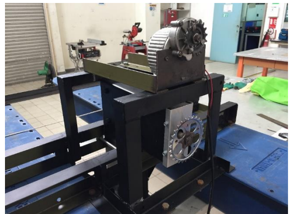
(b) Fabricated generator mounting plate.
