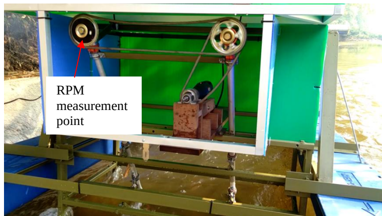
Figure 3.42: The prototype RPM measurement.
