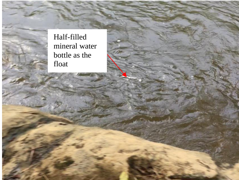
Figure 3.43: River flow velocity measurement with float method.
