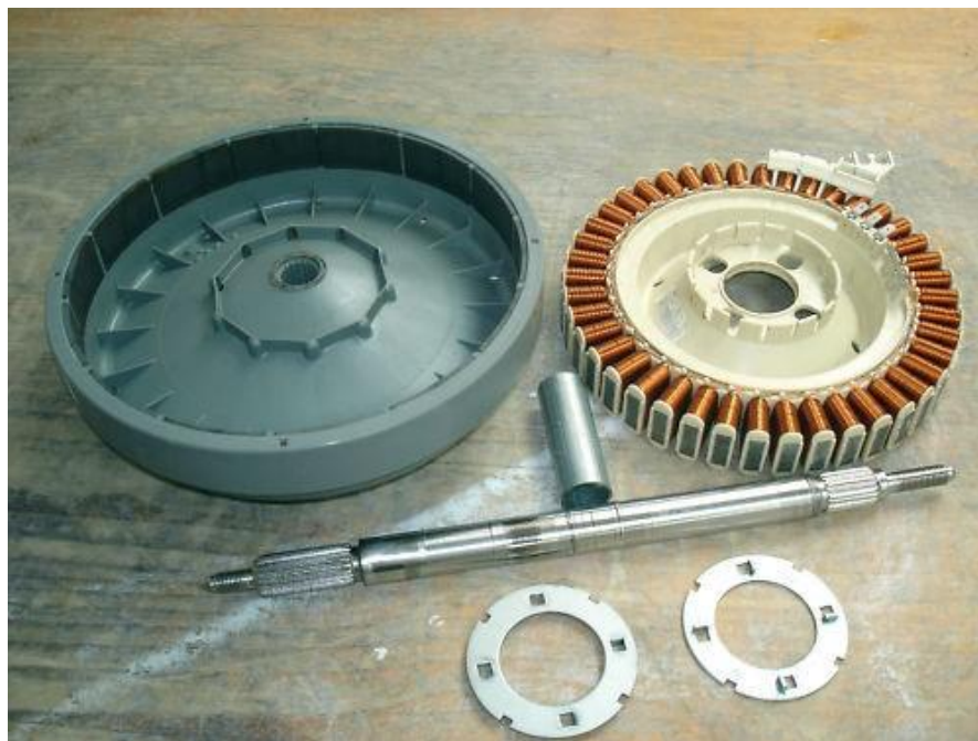
Figure 3.69: The 42-pole 60s Smart Drive motor.
