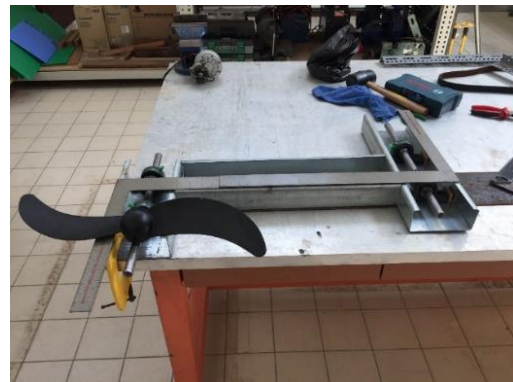
(b) Galvanised lip channel steel cut to size.
