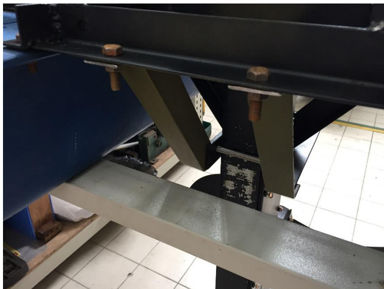
Figure 3.61: Rear supporting structure for the transmission.
