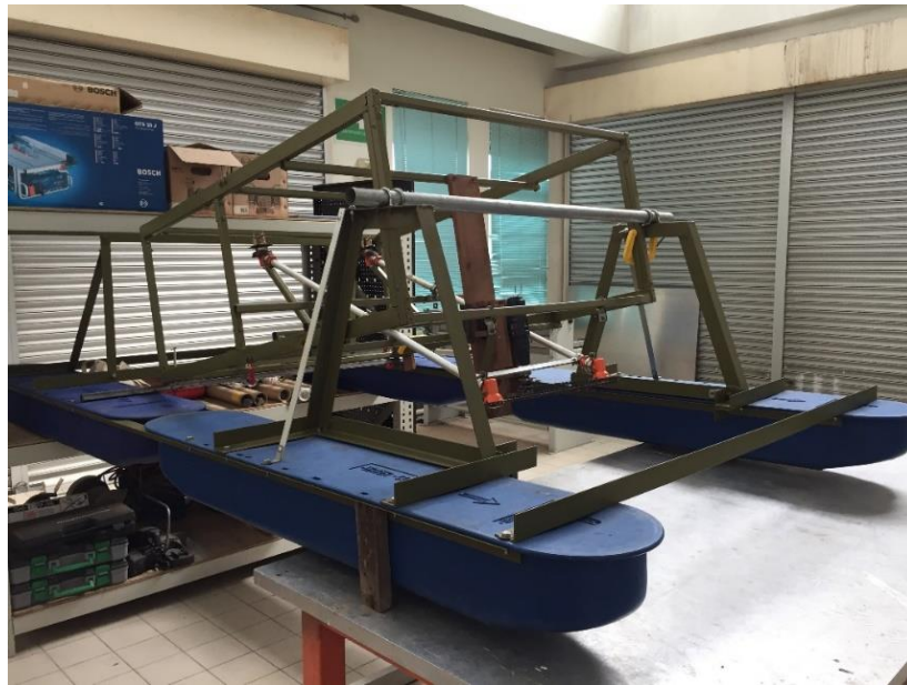
Figure 3.25: Constructed frame for winching.
