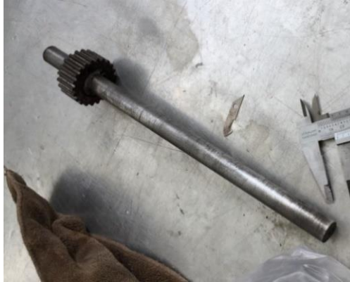
Figure 3.51: Pulley attached and welded to the shaft.
