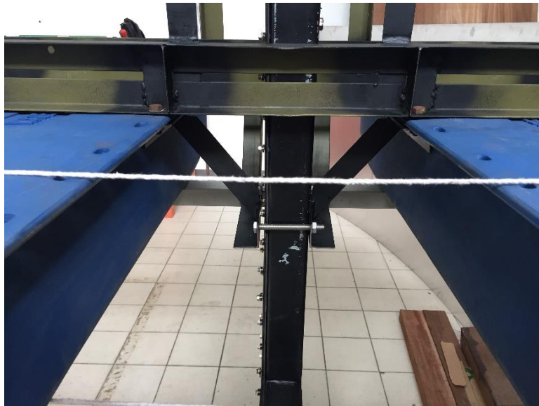
Figure 3.60: Side supporting structure for the transmission.
