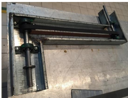
Figure 3.53: Galvanised lip channel steel trimmed and welded.
