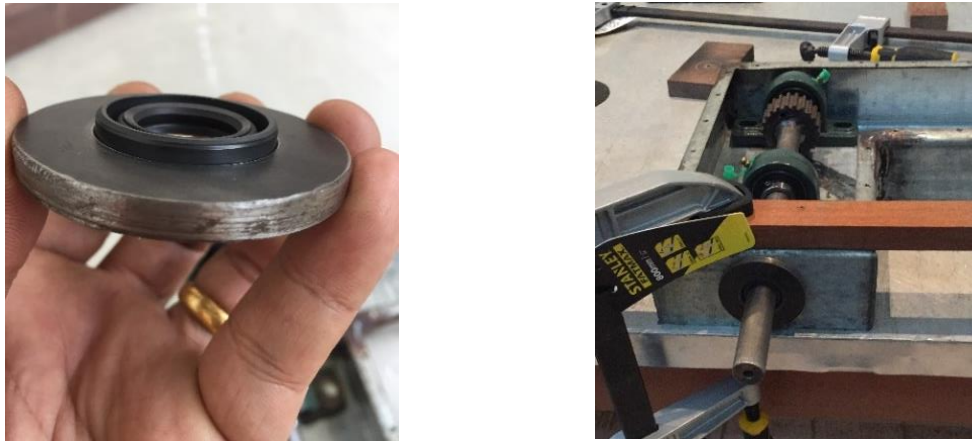
Figure 3.54: Oil seal attachment on the transmission casing.
