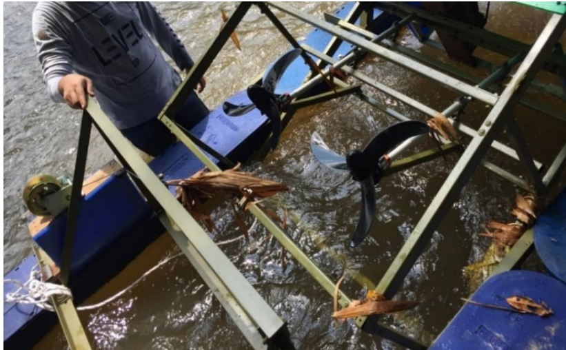
Figure 4.5: Submerged debris stuck on the turbine structure on day two.
