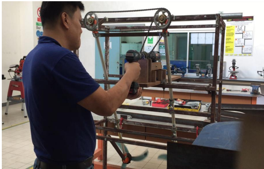
Figure 3.23: Testing the transmission with a cordless drill.
