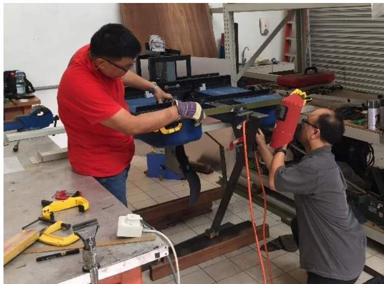
Figure 3.62: Front deflector cum leg fabrication.
