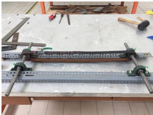
(a) The belt and pulleys layout.
