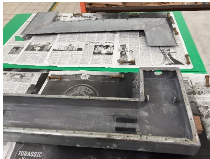
Figure 3.55: Casing coated with the anti-leaking sealant.
