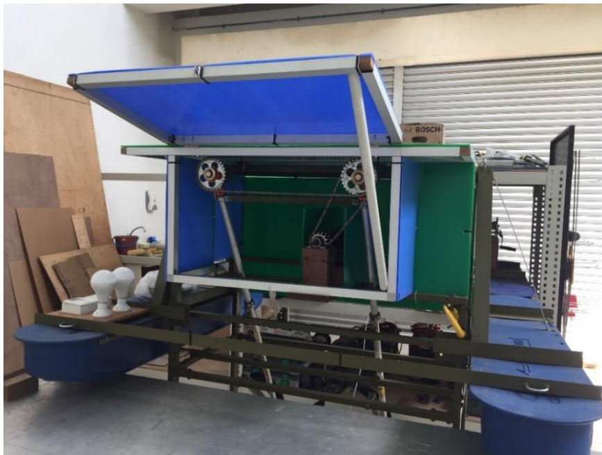
Figure 3.28: Fabricated cover for the swingable section.
