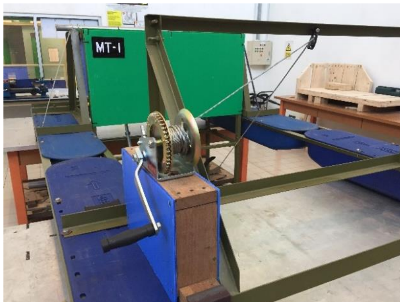
Figure 3.26: Hand crank winch and pulleys fixed to the frame.
