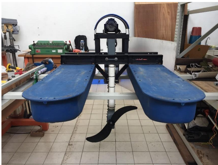
Figure 3.65: Completed improved prototype with leg structure removed.
