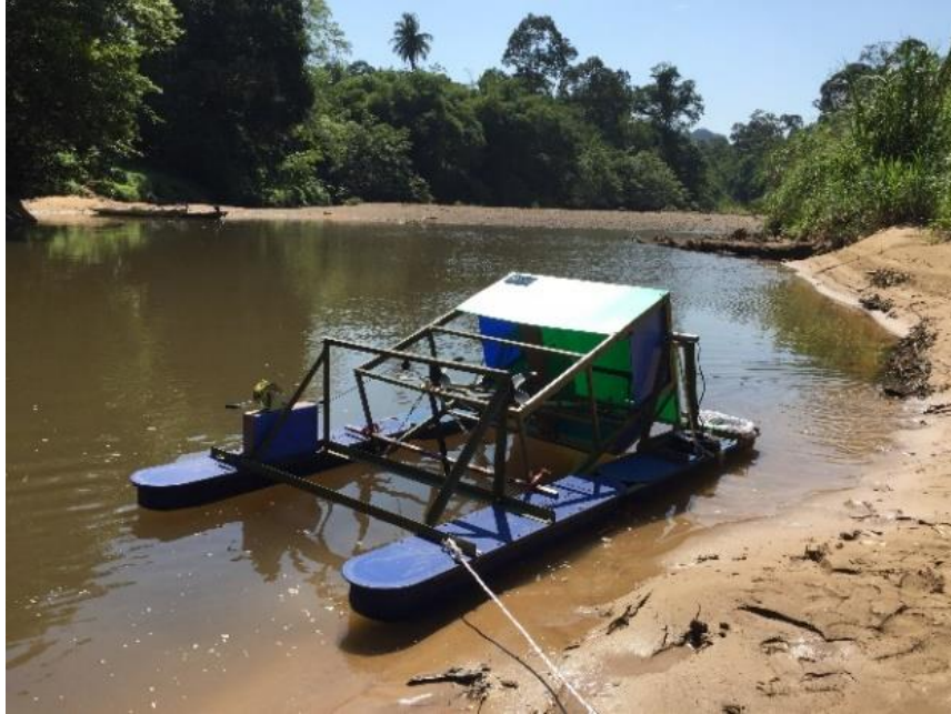
Figure 3.37: Testing the prototype buoyancy.
