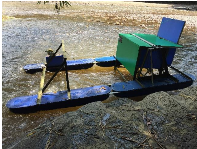
Figure 3.39: The prototype is secured to the testing position.
