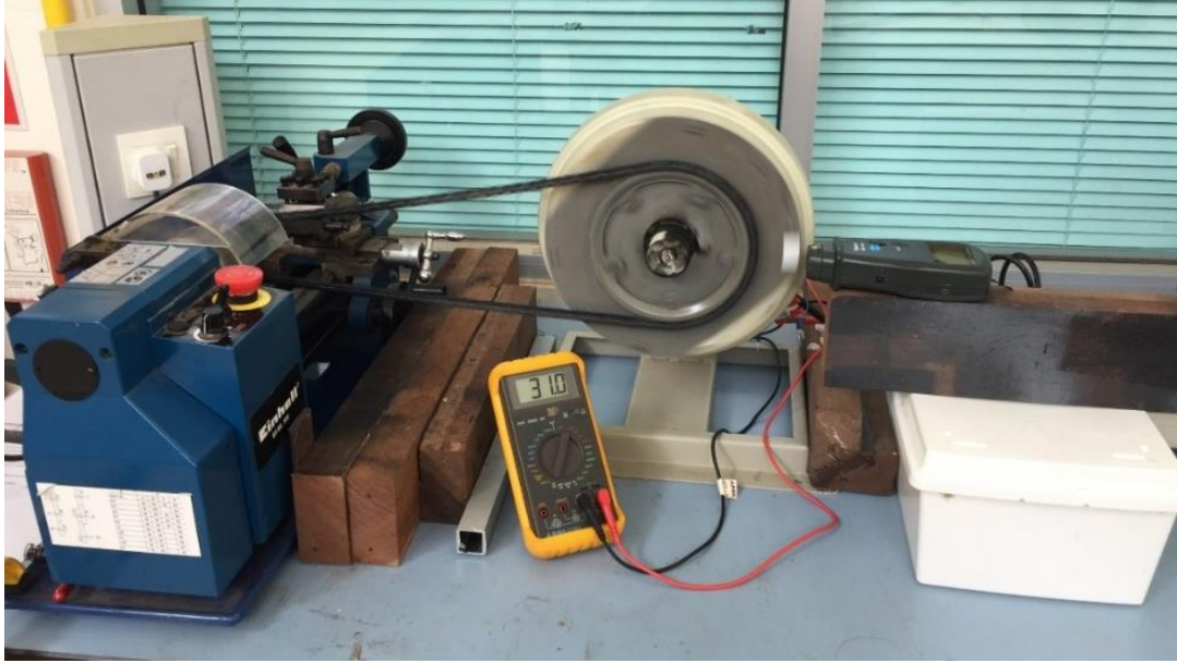
Figure 3.73: Testing the Smart Drive motor as a generator without load.
