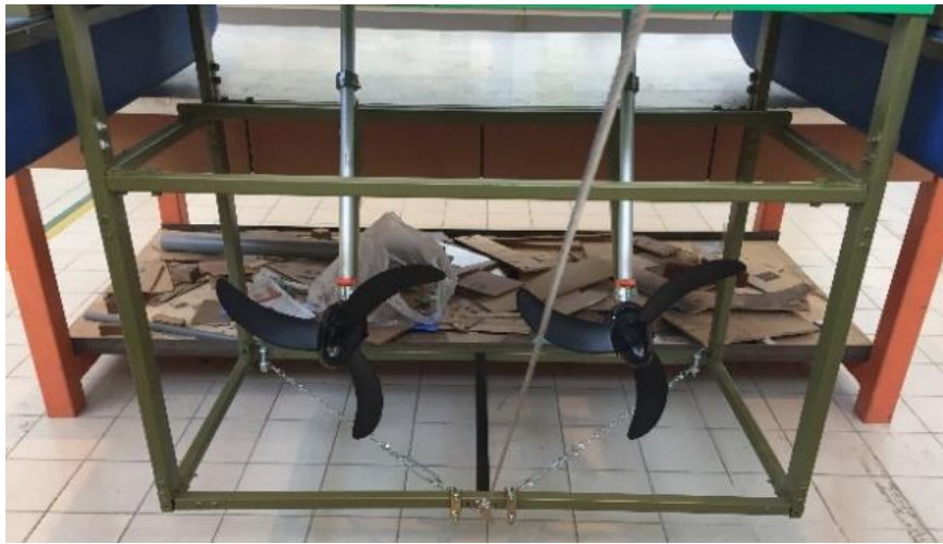
Figure 3.27: Fixing the steel cable to the bottom of the swingable section.
