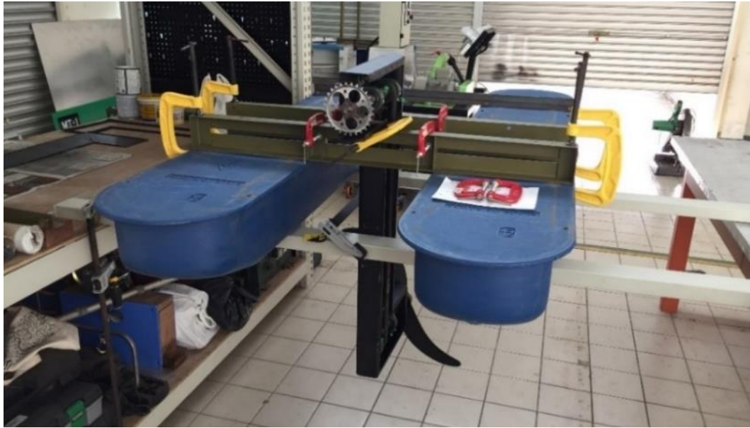
Figure 3.57: Fabrication of the transmission supporting structure.
