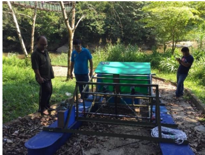
Figure 3.35: Lowering the prototype to the river using a ramp nearby.
