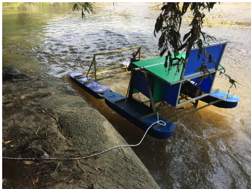
Figure 3.40: The turbine tilted as the river was shallow.
