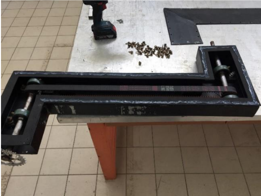
Figure 3.56: The completed first stage of the transmission.
