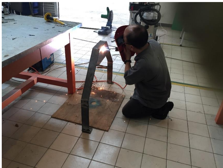
Figure 3.63: Rear leg structure fabrication.
