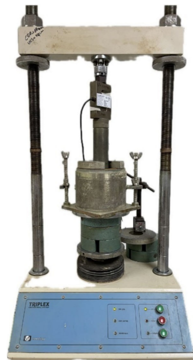
Fig. 7 Experimental setup of the CBR test
