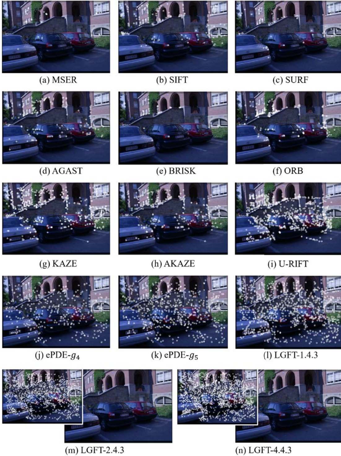
Figure 4.19: Comparison of inlier count and distribution in the stitched images of light-changed 'leuven' using different feature detectors. Inliers are marked by white circles and crosses. (m) & (n) include stitched images without markers for clarity
