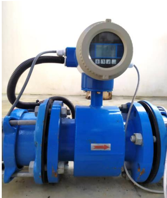
Figure 3.15: Inflow Electromagnetic Flowmeter
