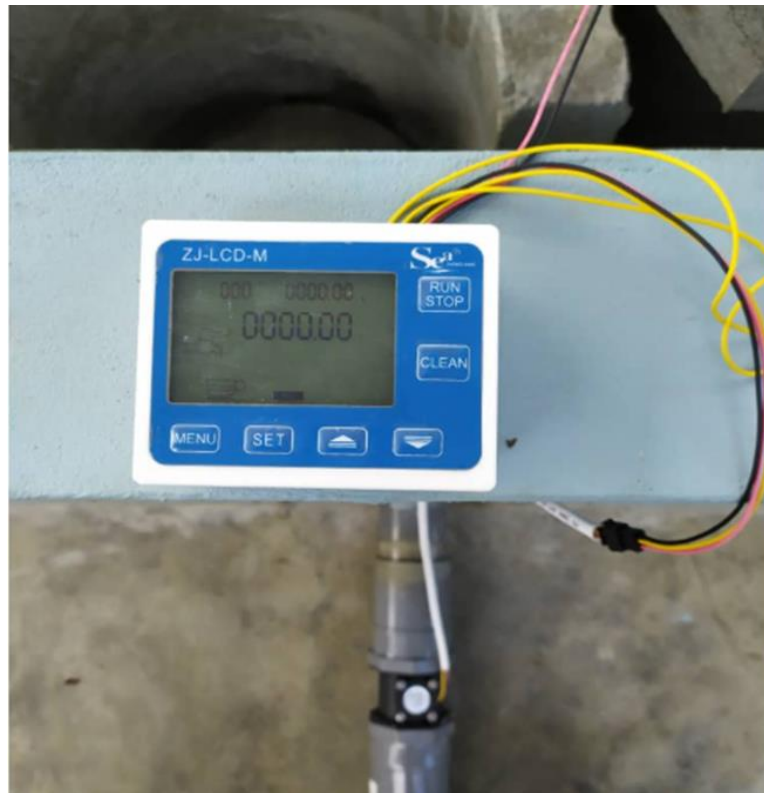
Figure 3.21: Outflow Electromagnetic Flowmeter
