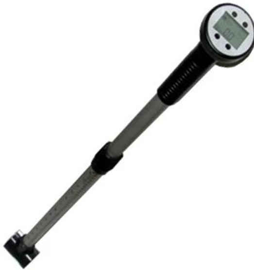
Figure 3.16: Water Flow Probe
