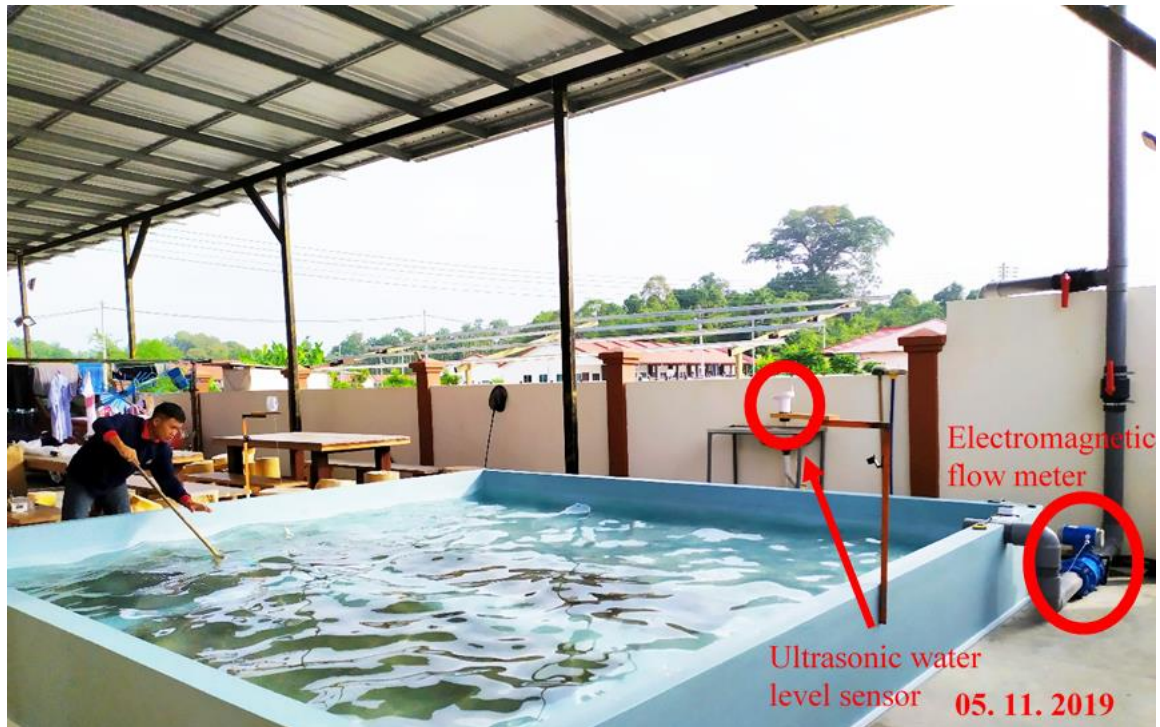
Figure 3.7: Water Leaking Testing of OSD
