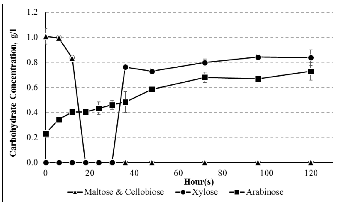
Figure 5.3: Time course of fermentable sugars such as maltose/cellobiose, xylose and arabinose concentrations, as determined by HPLC. [Note: The data points represent the average of three independent experiments (n=3).]
