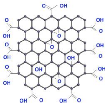
Figure 2.6: The Graphene Oxide (GO) structure. Image used with permissions of ACS Material ( https://www.acsmaterial.com )
