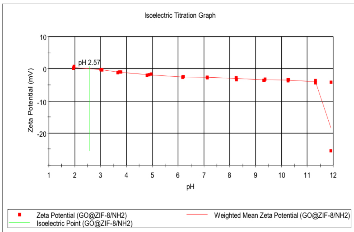
Figure 4.33: The isoelectric titration graph of ZIF-8/NH 2
